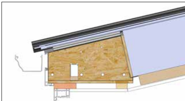
This image is showing the plaster line at 12.5° to 15° using 100 x 25mm timber packer (not supplied)
