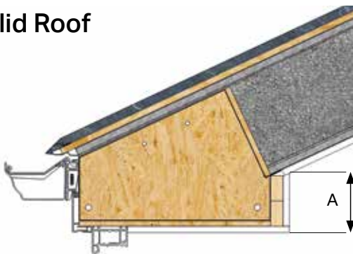
This image is showing the plaster line detail for a standard gable front. 44 x 70mm timber required above the gable frame.
